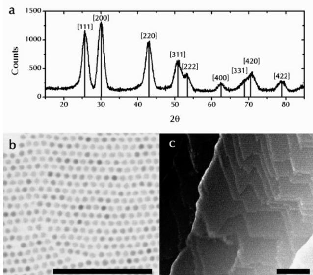
**Figure 1.** (a) PXRD of a PbS sample with vertical lines indicating the positions of the peak in bulk PbS. (b) TEM of a monolayer of PbS nanocrystals arranged in hexagonal packing; (c) TEM of a plasma-polymerized PbS nanocrystal superlattice obtained by slowly drying an hexane solution of nanocrystals and exposing the resulting film to plasma treatment.<sup>9</sup> Scale bars are 100 nm.
