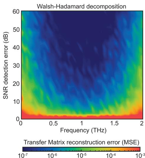
**Figure 2.** Transfer Matrix reconstruction. Mean squared error (MSE) of the coherent transfer matrix elements as reconstructed through a Walsh–Hadamard decomposition. The input and output planes are divided into  $16 \times 16$  pixels, corresponding to a scattering matrix composed of  $256 \times 256$  entries.
