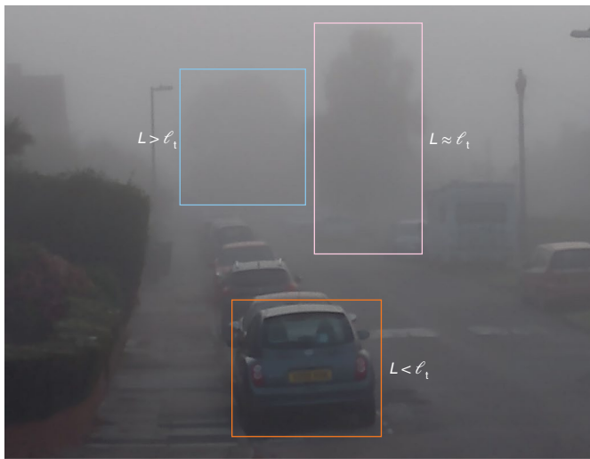
Fig. 1 | Imaging through fog as one example of optical imaging through complex media. Fog is composed of small water droplets that scatter visible light, preventing the formation of a clear image. Imaging through a layer of fog thinner than a characteristic distance, \ell_v , known as the transport mean free path, will result in a slightly degraded image, but if the thickness of the fog layer, L , is much bigger than \ell_v , no image can be formed at all.
