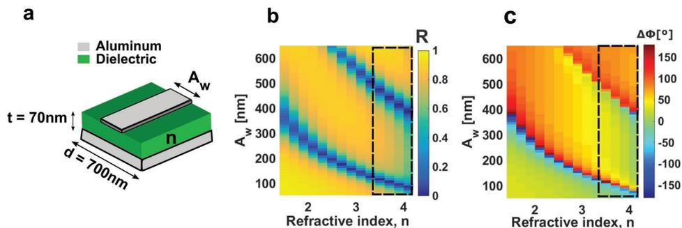
**Figure 2.** a) Generic MIM plasmonic resonator. Reflectance b) and phase c) as a function of the two variables: refractive index  $n$  and Aluminum patch width  $A_w$ . The dashed rectangle corresponds to the region where two resonant modes start to overlap (when  $n > 3.3$ ) and thus the target of a near  $2\pi$  phase control cannot be achieved.
