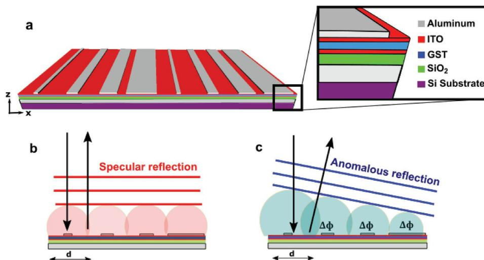
**Figure 1.** Reconfigurable phase-change beam-steering device design. a) Structure and materials of the device. Huygens principle showing the wave front reconstruction under normal incidence when the GST layer is in the crystalline b), and amorphous c) states.
