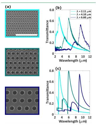
Figure 5. (a) SEM pictures of three laser-fabricated EOT metasurface devices with increasing geometrical periods (scale bar is  $10~\mu m$ ). (b) FTIR measurements of the fabricated samples, revealing a progressive increase of the transmission peak wavelength as the period increases. The results are in very good agreement with the numerical simulations shown in (c).
