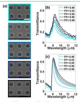
Figure 4. (a) SEM images of five different laser-fabricated EOT metasurface devices with different fill factors and identical geometrical period of  $\Lambda=6.6~\mu m$  (scale bar is 5  $\mu m$ ). (b) FTIR measurements of the fabricated samples, revealing a progressive increase of the transmittance as the fill factor increases, in line with the predictions by numerical simulations shown in (c).
